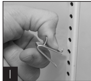
1 Installing top tab of shelf clip
