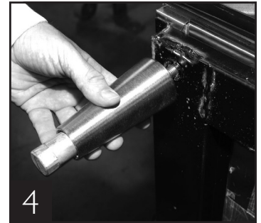
4 Thread leg into cabinet bottom frame rail.
