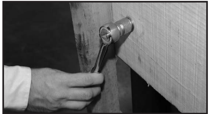
Removing skid from bottom of cabinet.
